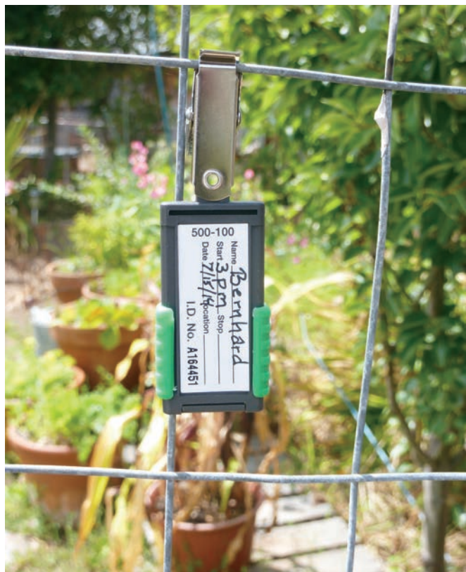
Formaldehyde badge clipped to an outdoor fence; a common air monitoring technique.
