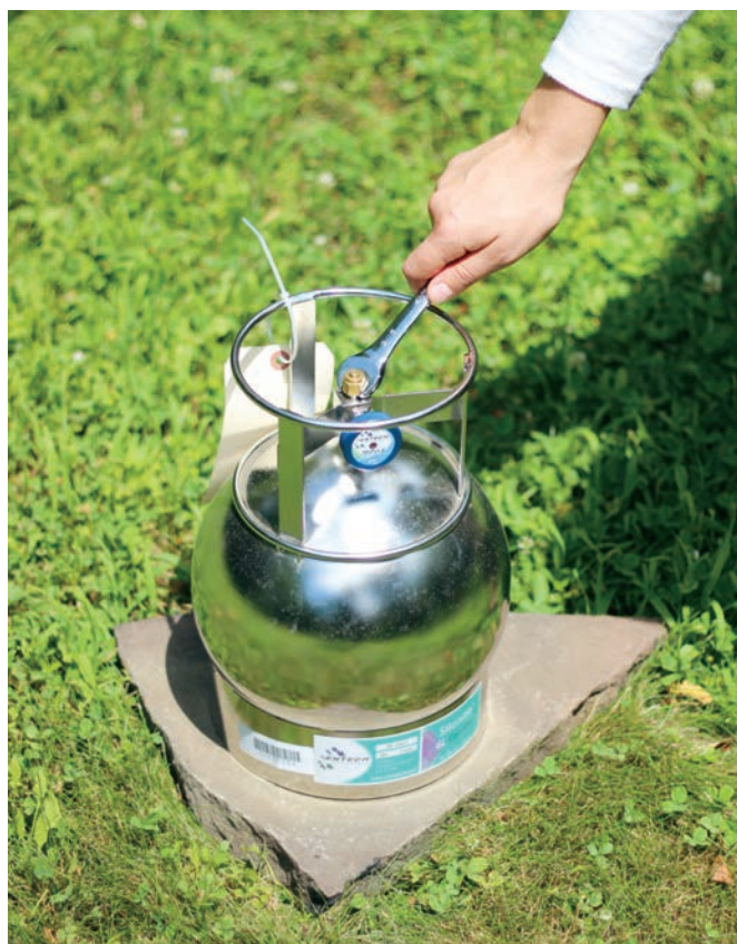
Summa canisters are frequently used by government agencies and communities to take air samples.
