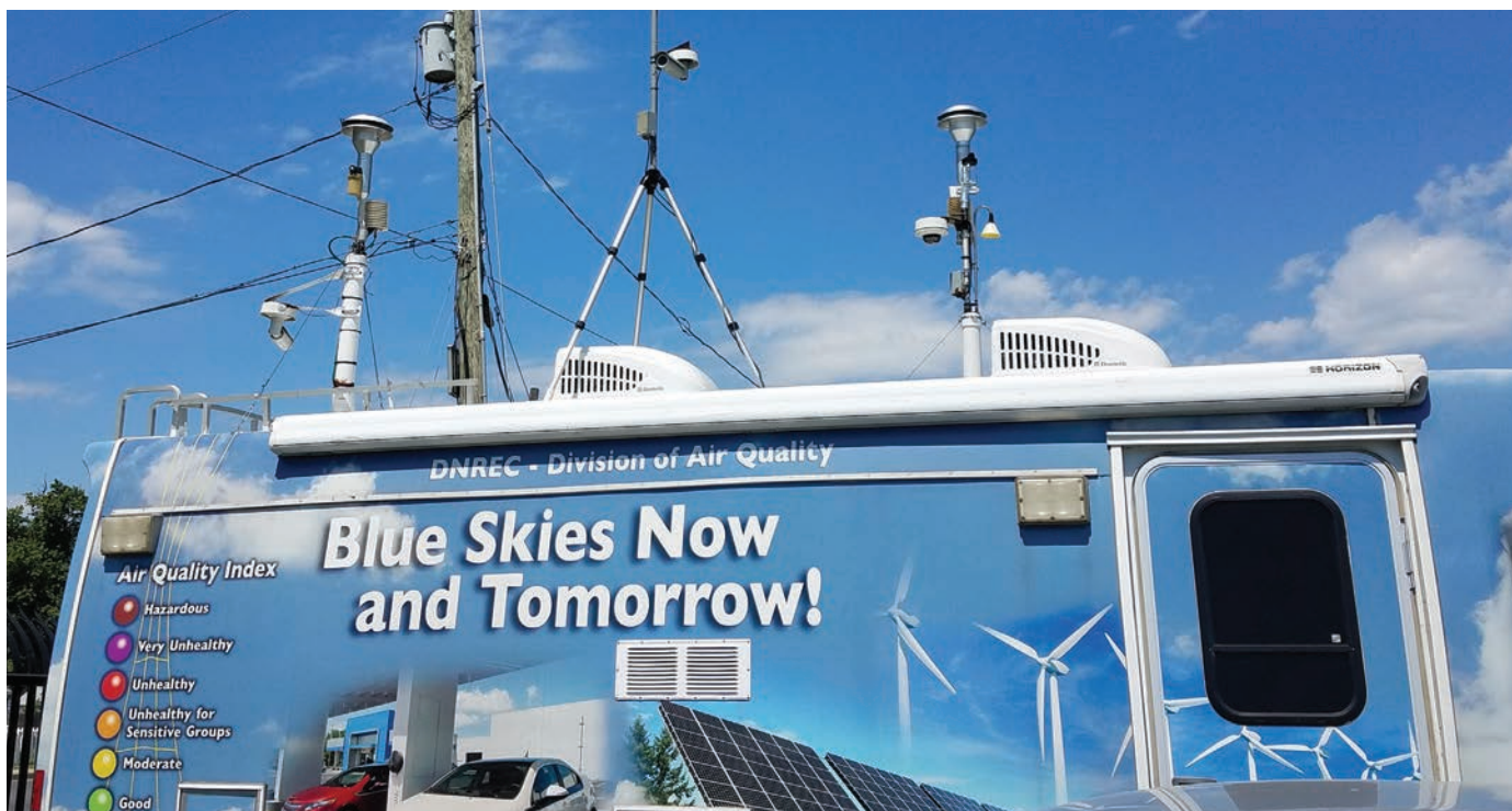
Mobile air monitoring stations like this one from the Delaware Department of Natural Resources and Environmental Control can allow communities to obtain air pollution data from locations without permanent monitoring but where pollutant levels may be high.
